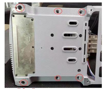
Turn over the machine like picture show and remove the foot base and 6 screws
