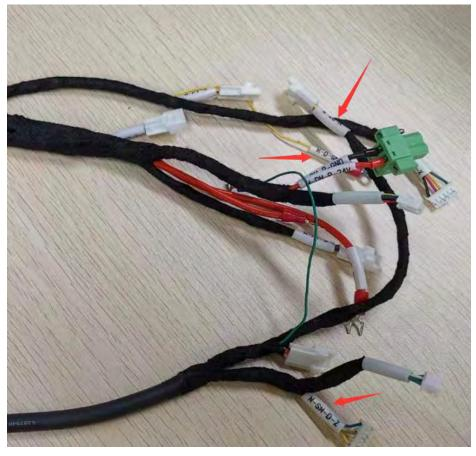
Left picture is the sensor and right picture are 2 cable cluster, it has mark for each small cable, insert every cable according to the mark also you can take some photos before you unplug the old cable
