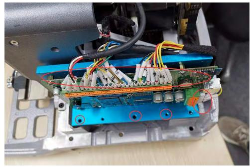
Unplug all pins on and 3 screws for remove the mainboard
