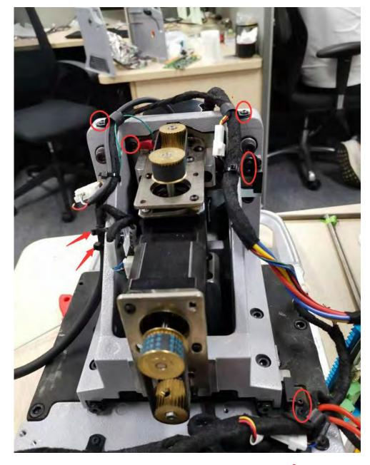
Take out the screws like mark it with red circle for remove the cable fixture and sensors, and also cut the cable tie for release those cables
