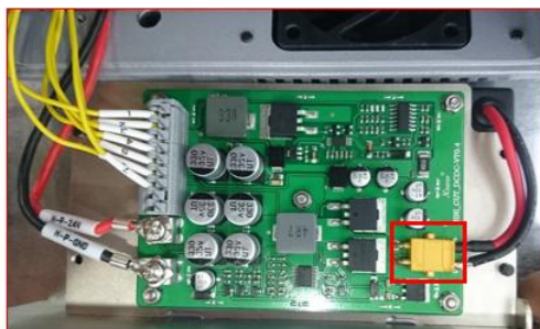
12, Connection the power like picture show then put back the Mainboard and fix it well
