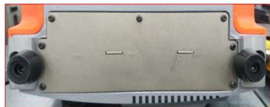
13, Fix the all cables after put back the mainboard , the mainboard should be in fixed very solid ,manage the cables again if not , then fix the foot rubber and screws
