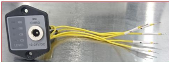
Battery charger & display module
