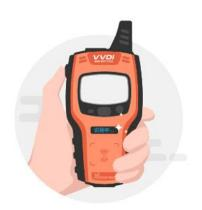
[Transponder detection]: press the power button for 1 second [Frequency test]: press and hold the power button for 2 seconds
