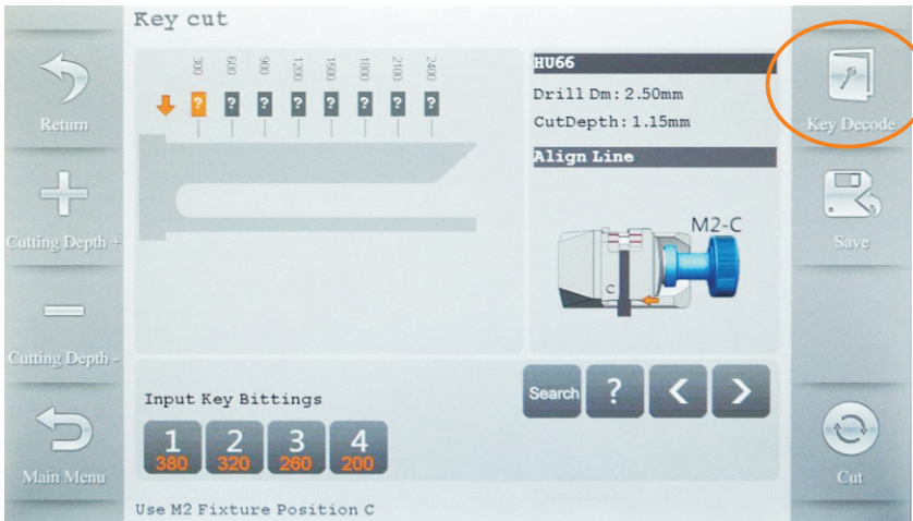
5 ) Put the original Key in the properly position of the clamp display on the screen, then Click on Decode Key
